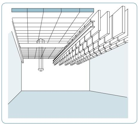
Sound-absorbing baffles help reduce reflected noise.
