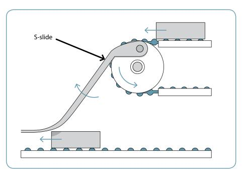
An S-slide will reduce drop height and deliver material quietly.
