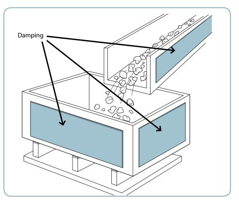
Installing damping in delivery chutes and bins will reduce noise.
