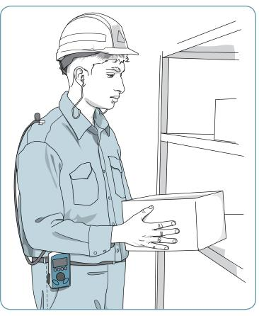
Workers wear noise dosimeters over the shoulder or on the collar.
