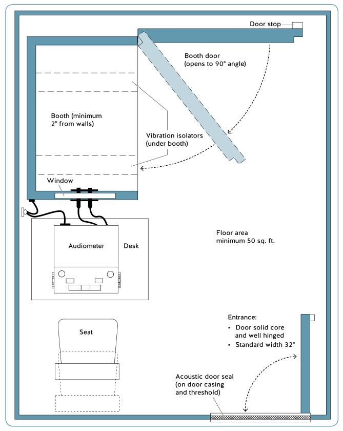
Requirements for hearing-test facilities are specified in the WorkSafeBC publication Industrial Audiometric Facility Approval Process and in CSA Standard Z107.6-16.
