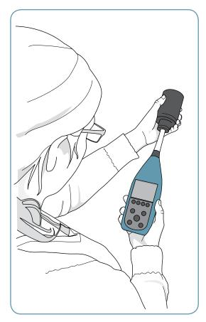
Integrating sound level meters average noise levels over time. To ensure proper function, these should be calibrated before and after a survey.
